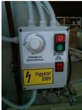
Heating can be started with the red toggle switch under the main switch. This starts the pump motor which circulates the water as well. The water temperature is adjustable. Based on our experiences, a water temperature of ca. 55°C degrees is ideal, which increases the efficiency of uncapping, but does not cause changes in the honey.
