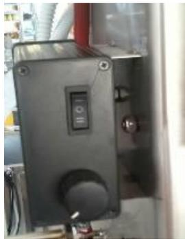
Additional switches are provided on the right side of the automatic uncapper viewed from the front. The lateral movement of the knives can be started with the vibration switch. Their speed is not adjustable.
