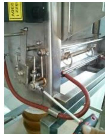
The screws helping the lateral fastening of the frames are located under and above the switch activating the pulling of the frame (indicated by an arrow on the image). Loosen the screws to increase the lateral tightening of the frames, and tighten the screws to reduce it. (the frames will move more easily)
