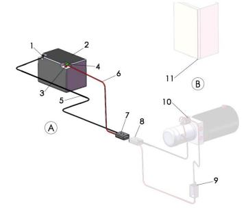
As for the power of the crane, you should only worry about making connections corresponding to the area of the vehicle (A), as the crane (B) is sent fully equipped.
